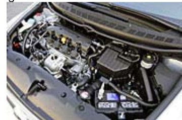
The 2007 Civic GX uses a 1.8-liter, four-cylinder engine with 113 hp and 109 ft.-lb. of torque.
